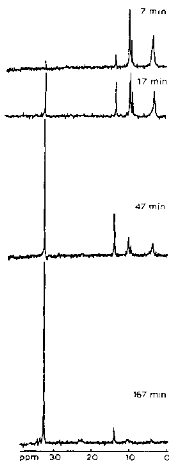
Fig. 6. ^{31}\text{P} NMR signals vs. time for the reaction 0.05\text{ M } \text{tn}_2\text{CoP}_2\text{O}_7^- ( \delta = 4\text{ ppm} ) with 0.1\text{ M } \text{tn}_2\text{Co}(\text{OH}(\text{OH}_2))^{2+} in 1.0\text{ M} TEA buffer at \text{pH} = 7 , T = 25^\circ\text{C} (Scheme 3).
